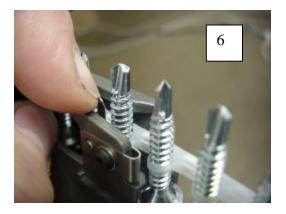
If difficulty is experienced, check that the strip is not stuck on the feed latch. The strip spring may be held back with one finger (photo 6), while the strip is removed. Wiggle the strip while withdrawing if required.
